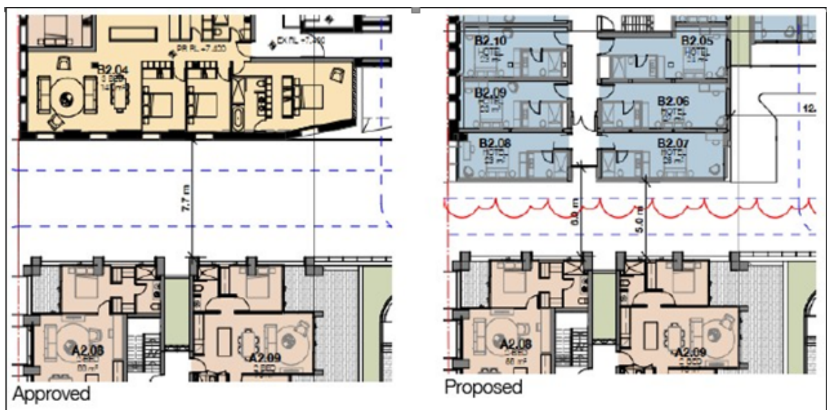
Figure 6: Building separation between Building B (top) and Building A (bottom), Level 2 Left: Stage 1 as-approved DA; Right: as proposed (Source: Figure 26 of SEE, SJB Planning)
